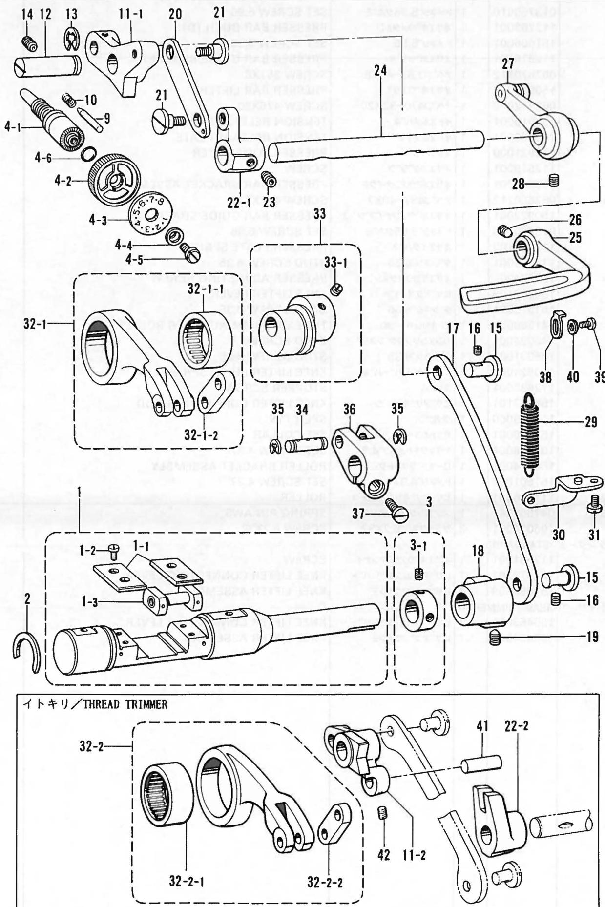
F. 送り関係/Feed mechanism/Transportvorrichtung/
