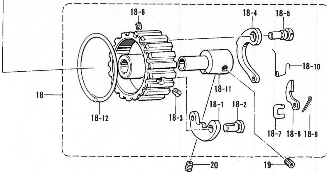
K. 下軸関係/Lower shaft mechanism/Untere welle/
