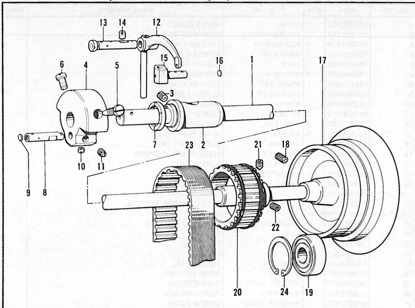
C. 送り軸関係/Feed shaft mechanism/Transport welle/
